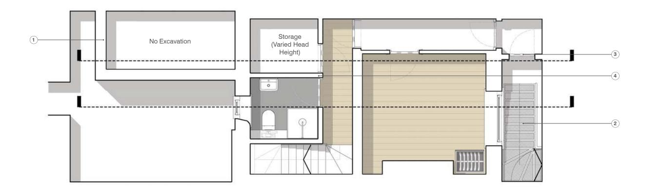
BASEMENT FLOOR PLAN. DRAWING no. 2000/D 1:50@A3
