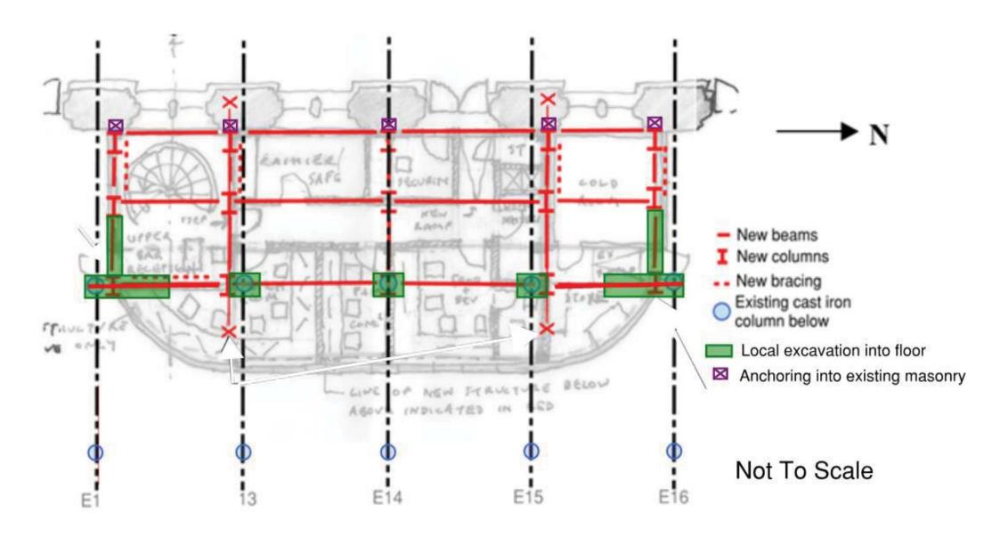
Figure 8 - Plan of new structure with excavation and anchoring locations shows the approximate locations where the cutting into the existing masonry floor is proposed to accommodate the detail in Fig. 7.
