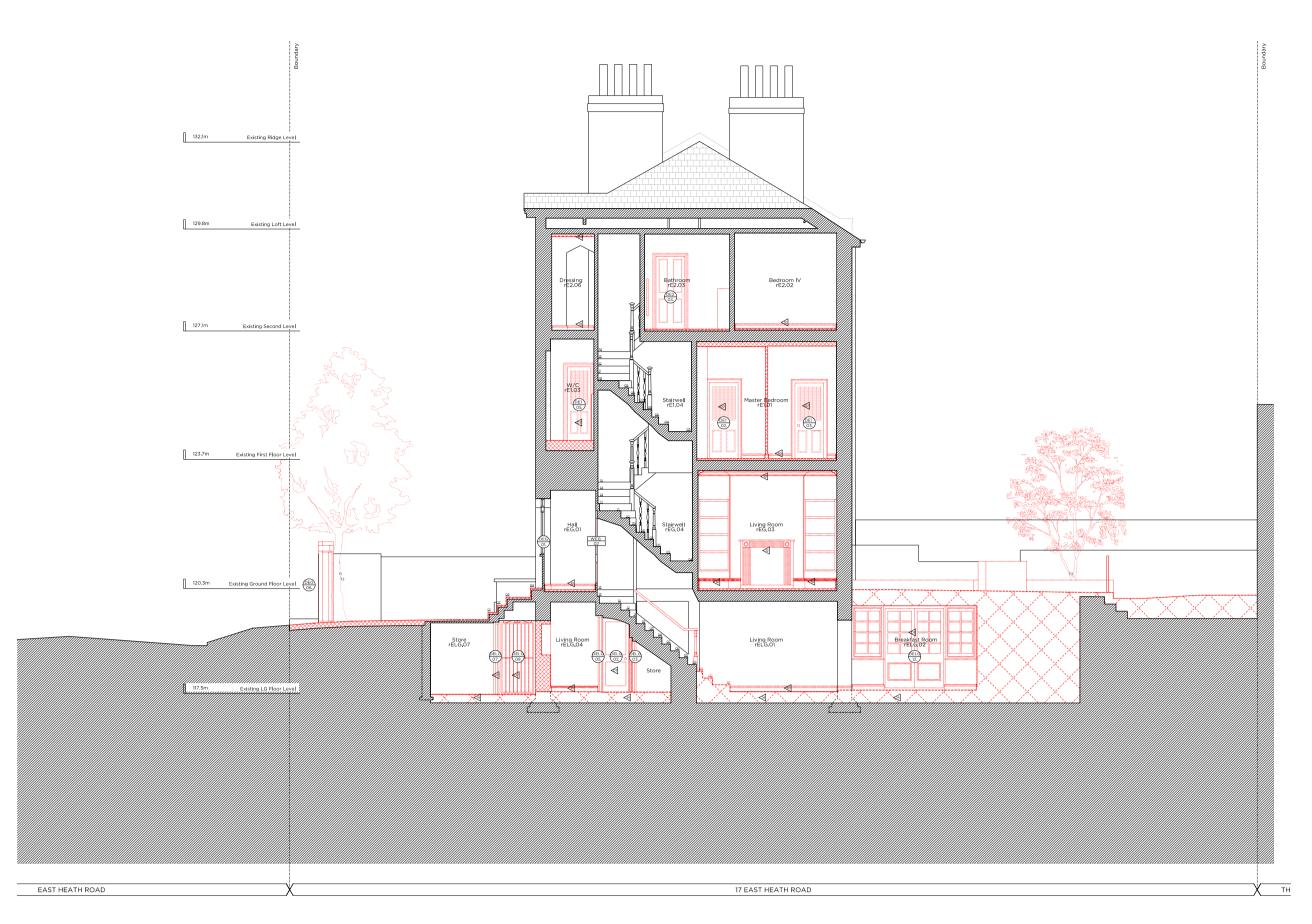
Existing structure / fittings to be removed Hatch denotes area of excavation New Soll Hatch denotes area of gardening excavation ---- Line denotes removal of existing structure
