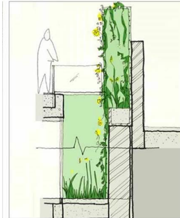
Sketch: Planted trellis A new boundary wall is built against the existing garden wall. A trellis allows planting to grow up and over to provide a similar level of privacy as currently enjoyed. Suitable planting will encourage biodiversity to the site.
