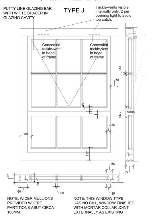
Do not scale from this drawing All dimensions to be checked on site Notes: Rev #. First Issue. 2016-07-20 Rev B. Trickle vents altered. 2016-11-01 Drawing type: L. B. CAMDEN Project: **LEVITA HOUSE EXISTING AND PROPOSED** WINDOW TYPE P Scale: 1:10@A3 Date: 27/10/2016 Drawn: JMA Checked: SB Drg.no: 5675-A(31) TYPE J Heritage Surveys Ltd. Heritage Surveys Limited 20 Hanover Square London www.heritage-surveys.com
