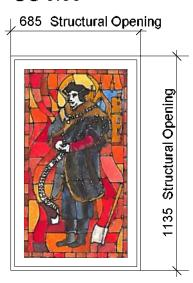
Thermally broken aluminium frame, polyester powder coated with double glazing. Colour to be RAL 7016.
