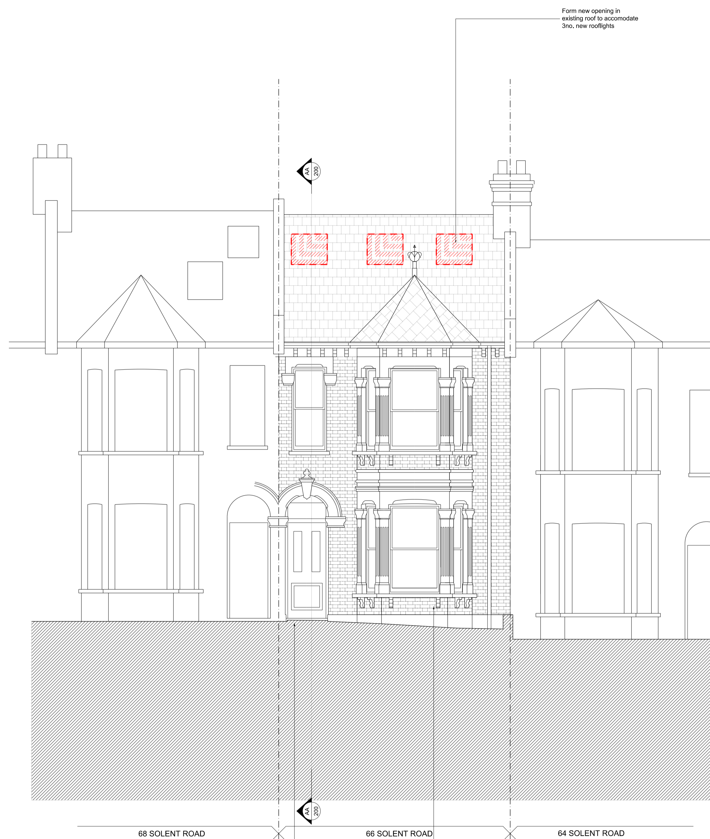
EXISTING & DEMOLITION FRONT ELEVATION
