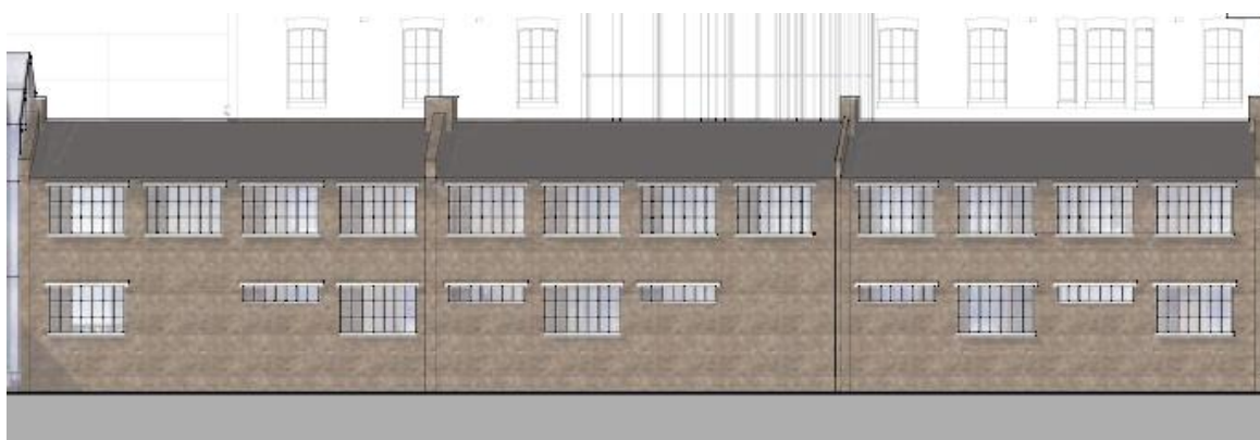
Figure 7 – Refurbished Commercial & Residential Unit Windows – Railway Facing Elevation
