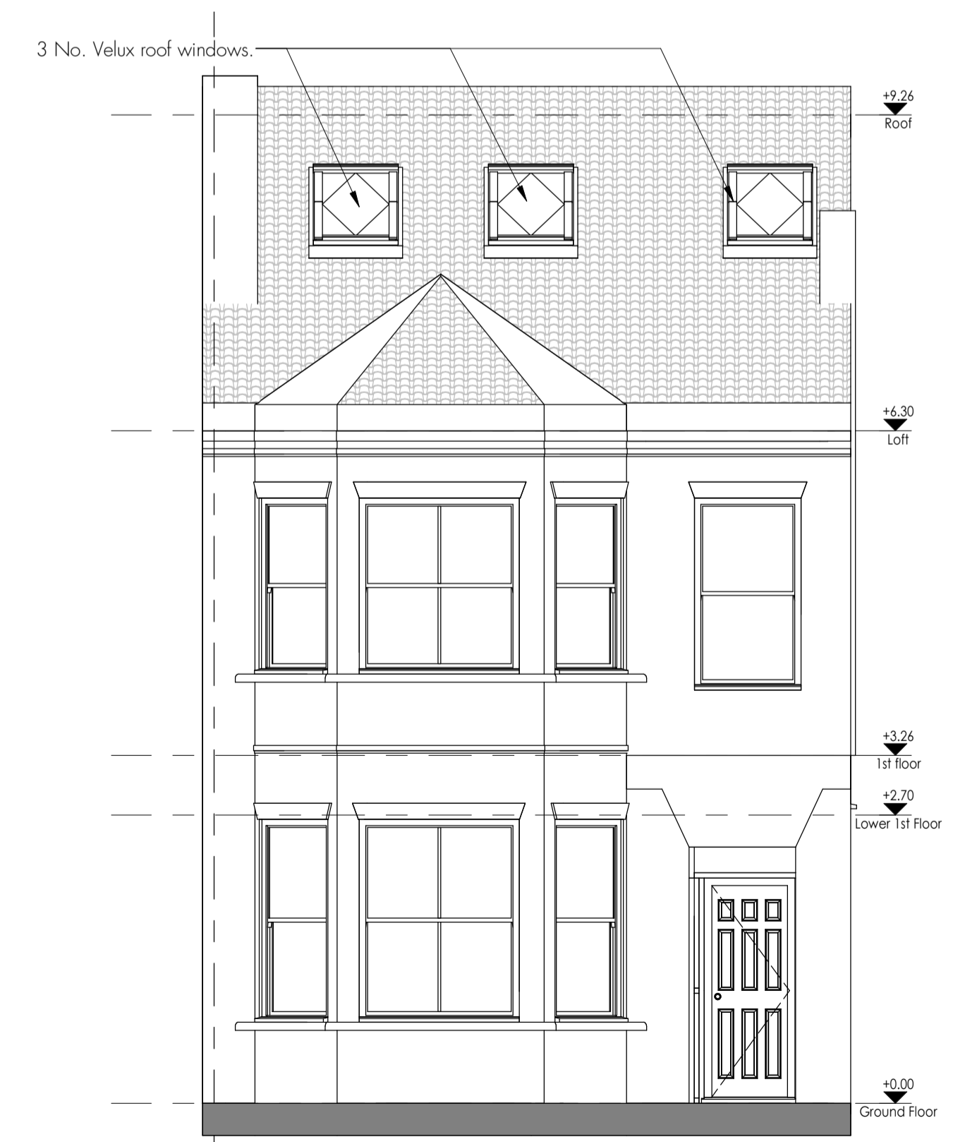
No. 5 | No. 6 4 Existing Front Elevation 1 : 50
