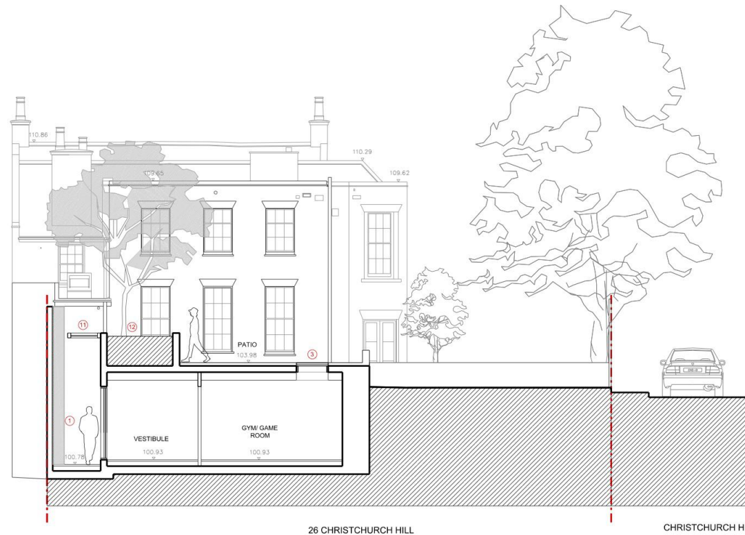
diagram 9 – section through basement area and 'sunken' courtyard with traditional construction method
