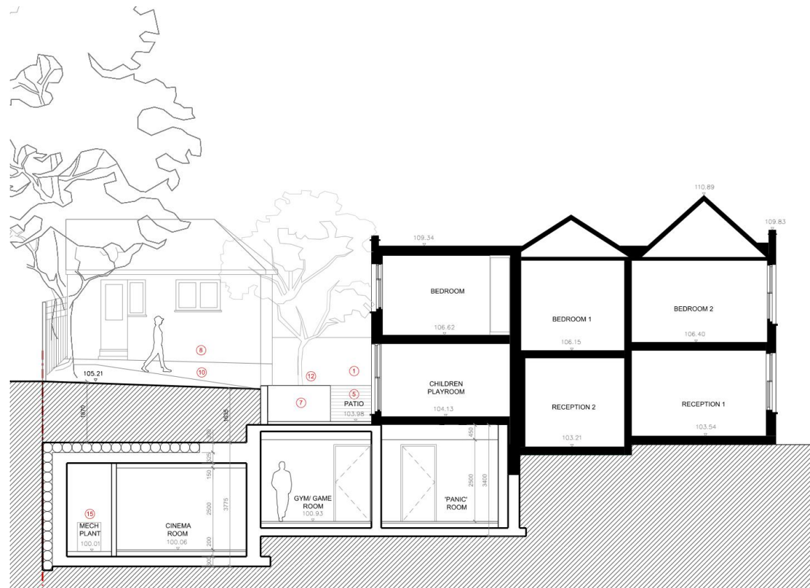
diagram 9 – section through basement area and 'sunken' courtyard with traditional construction method
