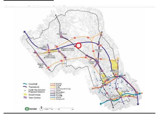
From Figure 18, Arup Report, and from maps of the local area. The Thames link rail line runs west / east just directly to the north of the property. However the depth / proximity of the tunnel will not have any influence on the basement.
