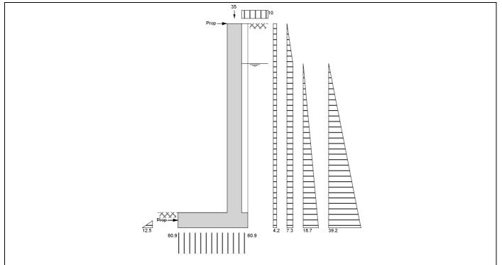
Loads shown in kN/m, pressures shown in kN/m $^2$
