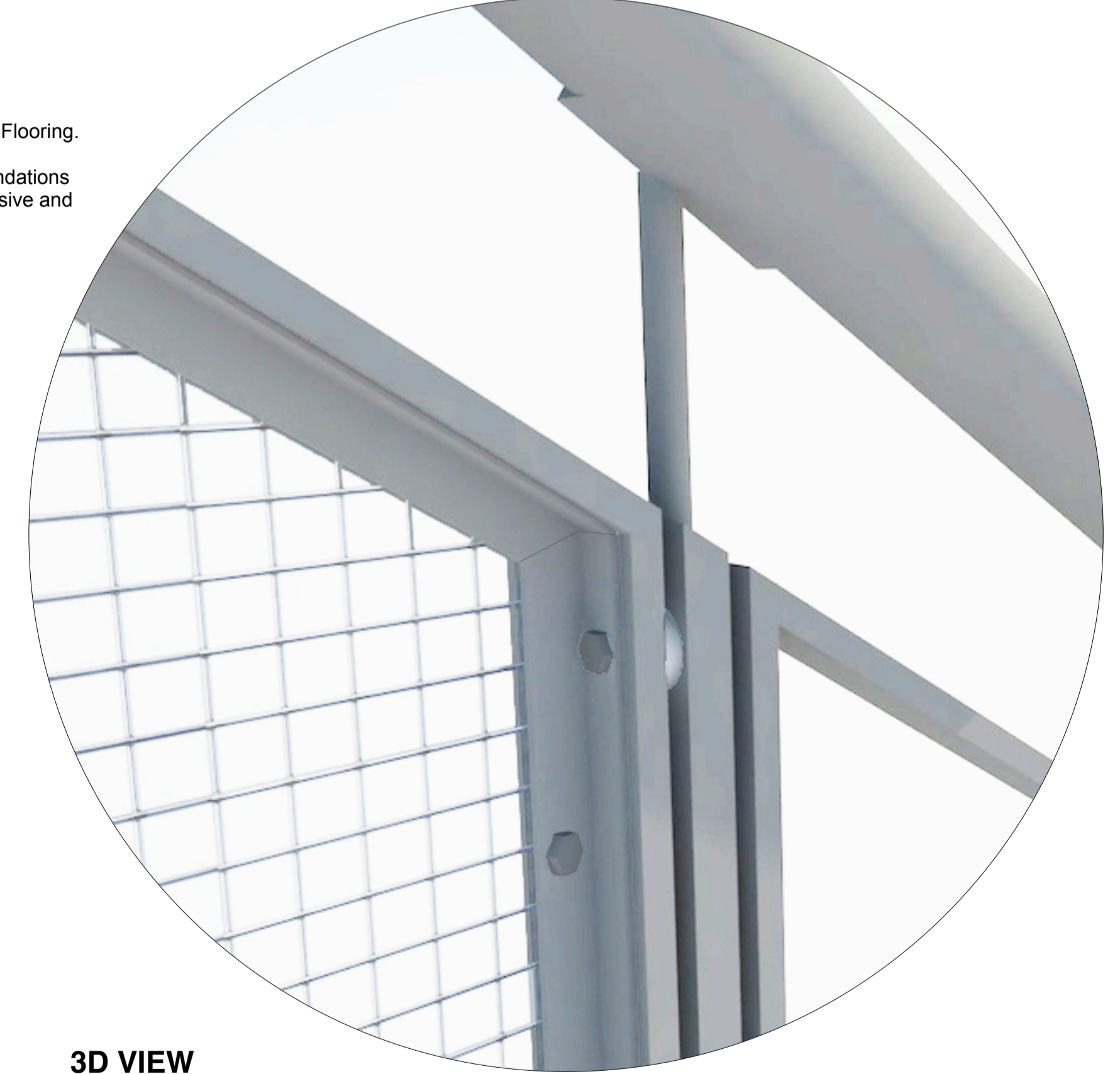
TYPICAL MESH FIXING DETAIL AA 1:1 @ A1
