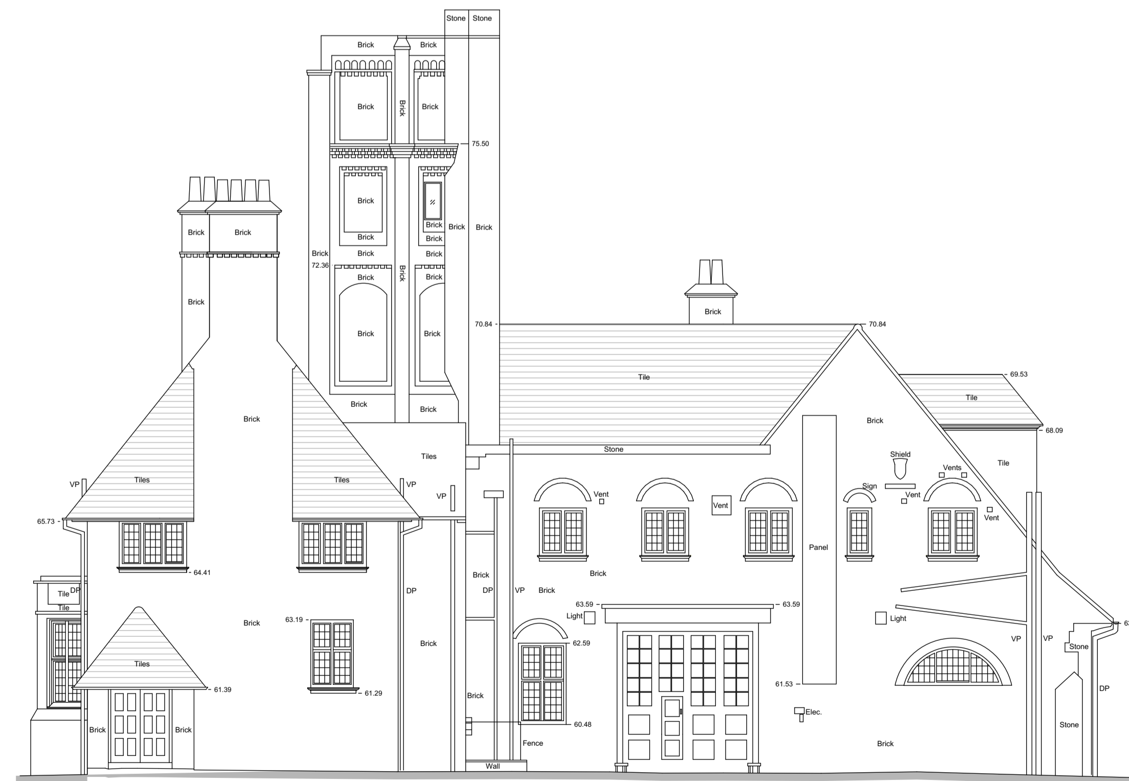
EXISTING EAST ELEVATION
