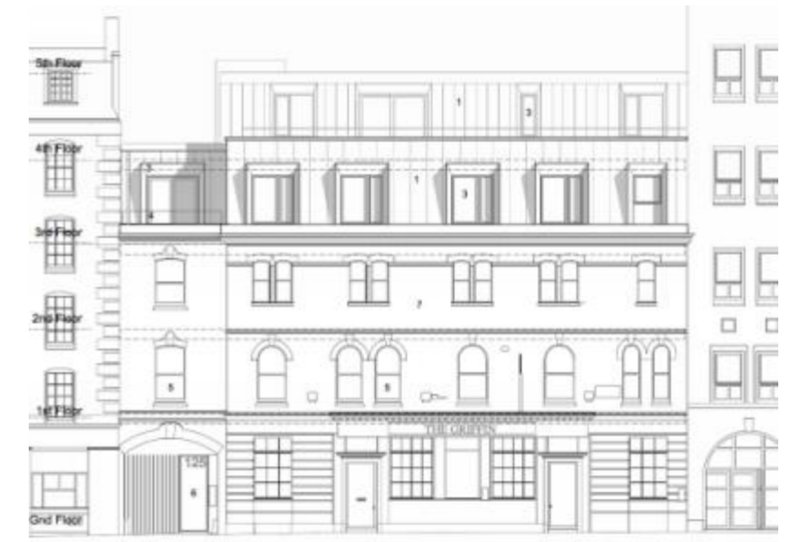
North facing glazing has been reduced on the top floor following Passive design considerations.
