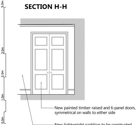
New lightweight partition to be constructed with replica skirting and cornicing instated
