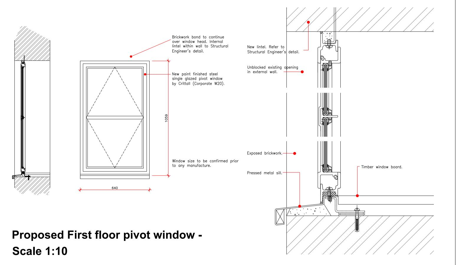
Proposed First floor pivot window - details Scale 1:2
