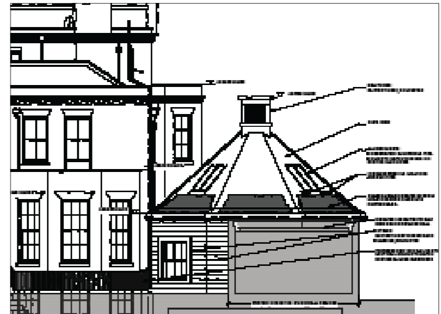
Partial elevation showing possible solar slate locations
