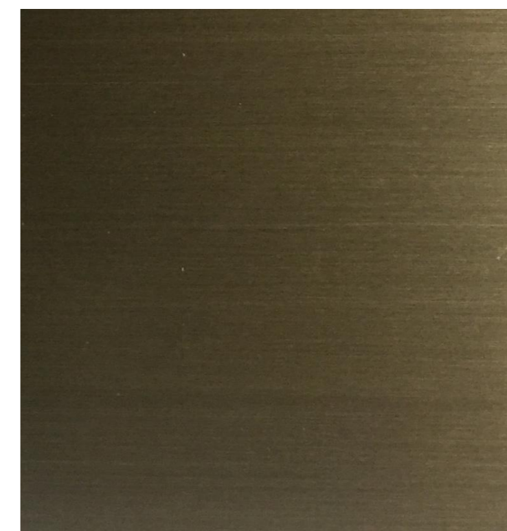
above Proposed finish for the new Portico Doors Sample provided by proposed fabricator Stewart Fraser Finish 'Antique Bronze Patina'
