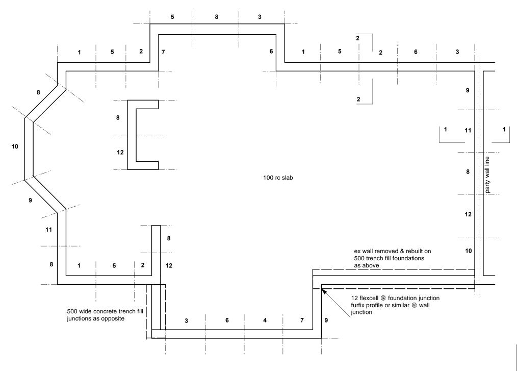
underpinning sequence as shown also refer to specification minimum depth of trench fill to be 1000 & to DS requirements party wall matters are to be noted
