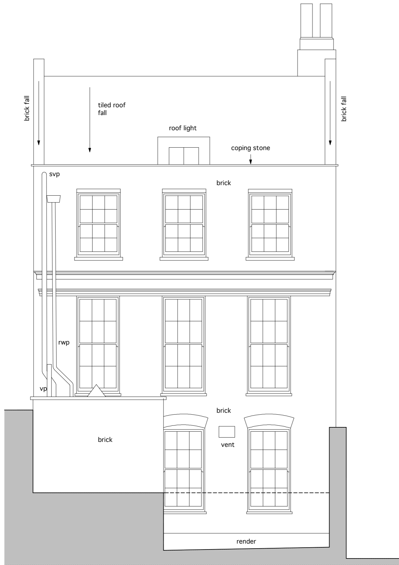
EXISTING REAR ELEVATION
