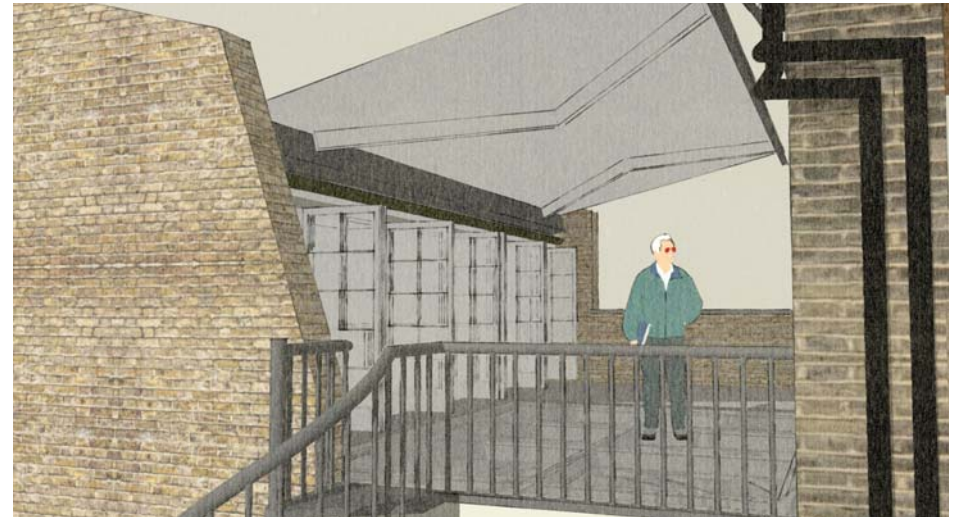
Retractable canopy to terrace, mounted on annex structure.
