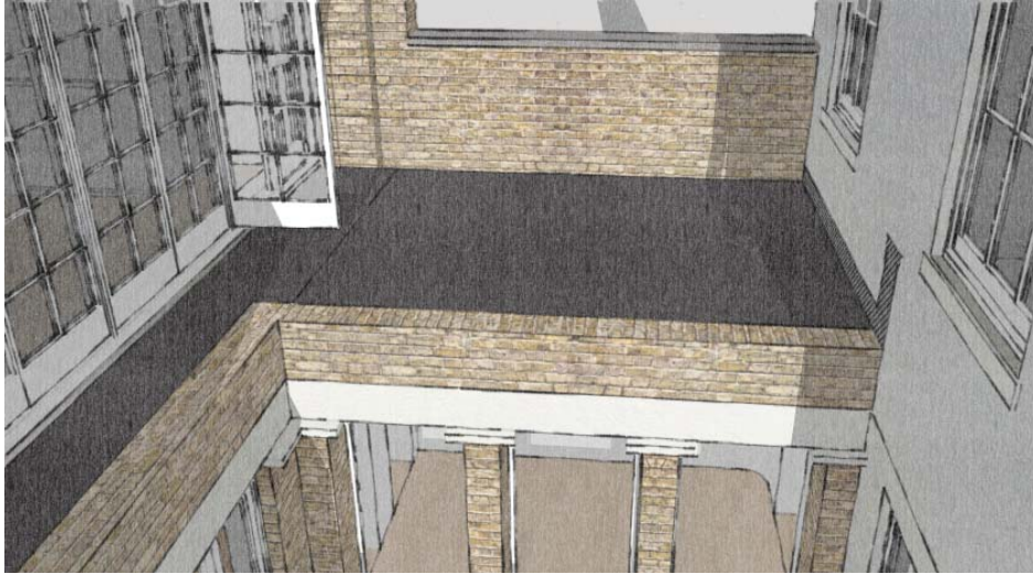
Up stand to link roof removed.
