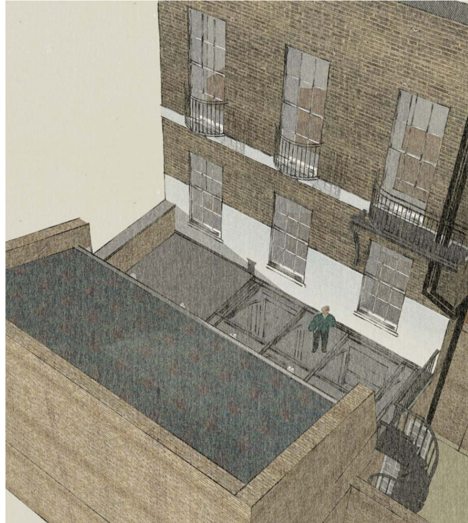
Sketch view looking into rear courtyard showing new glass floor above proposed garden room. Rear facade of No 1 shown.
