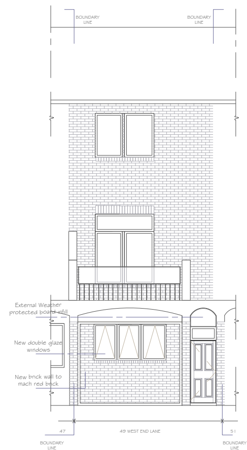
PROPOSED WEST END LANE ELEVATION PROPOSED FRONT ELEVATION
