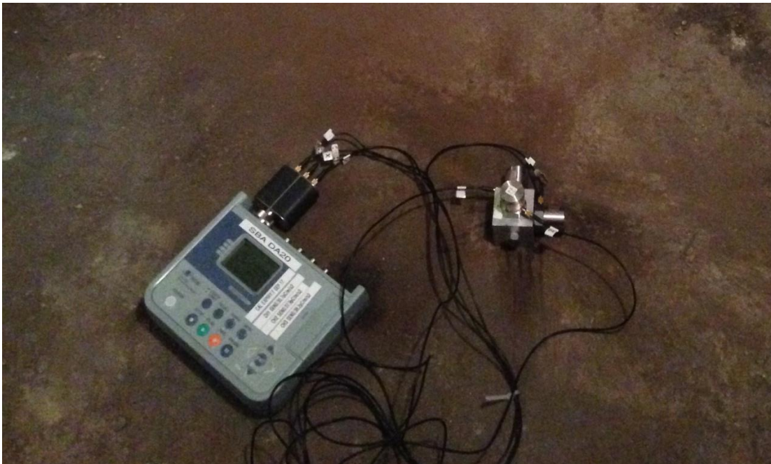
Figure 3 Photograph of vibration measurement equipment set up
