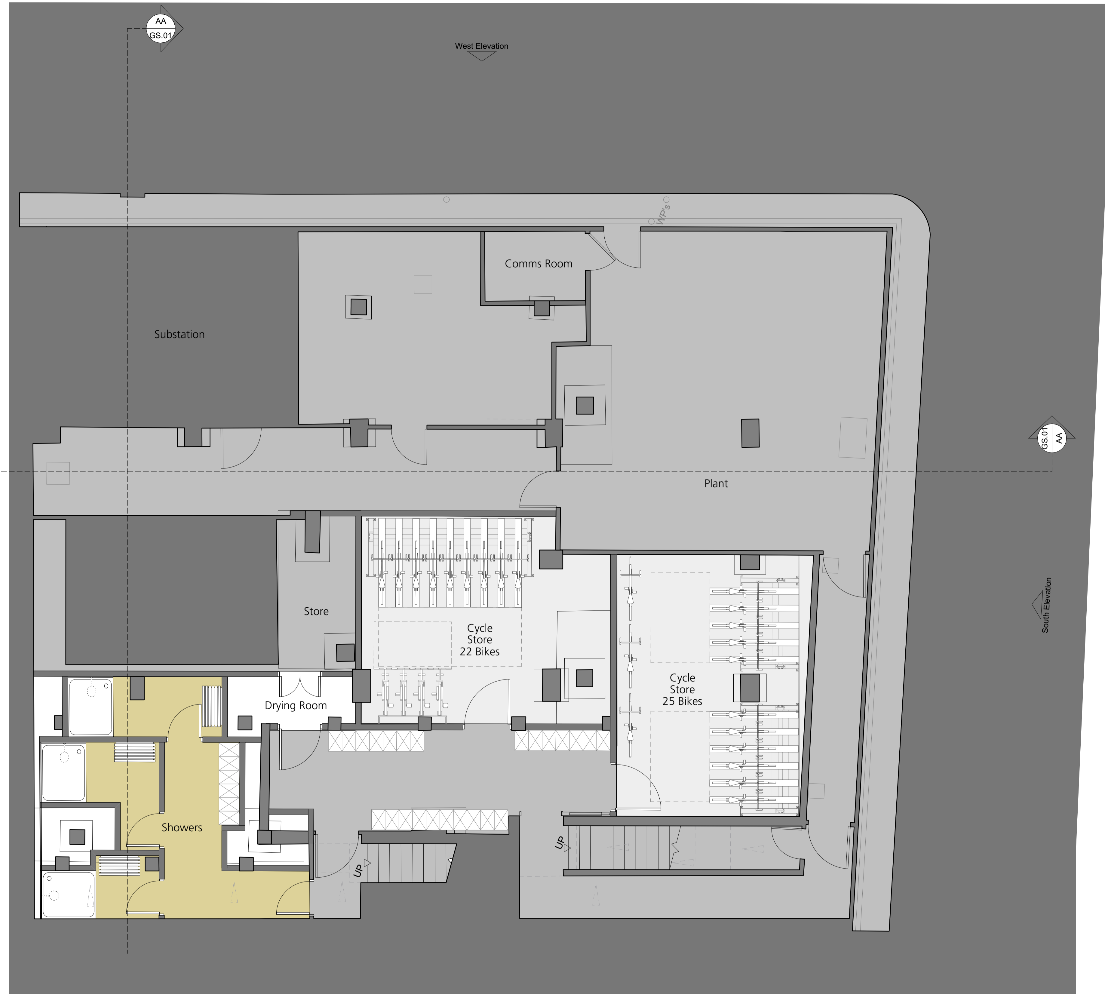
1 Proposed Basement - Op2 Scale: 1:50
