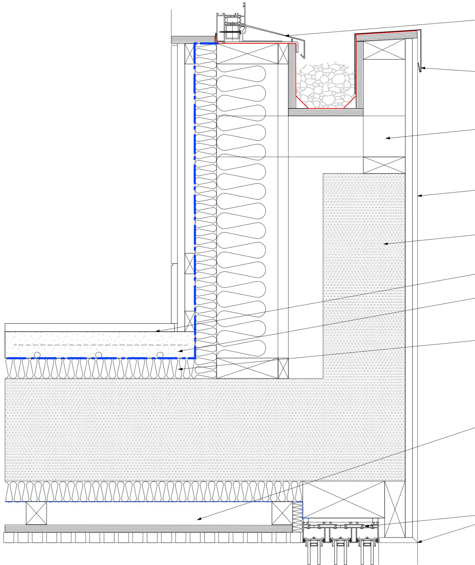
Pivot / fixed glazing with cill detail to allow for water runoff into gutter in powder coated aluminium by specialist. Thermally broken profiles & low e double glazing to give U value of 1.4 W/m2K.. Refer to Window Schedule for further details.
