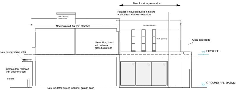
Proposed Section X-X & East (Side) Elevation
