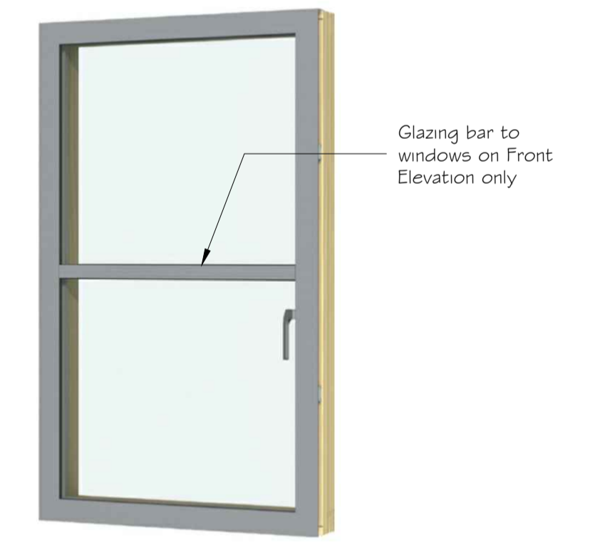
TYPICAL WINDOW (external view NTS)
