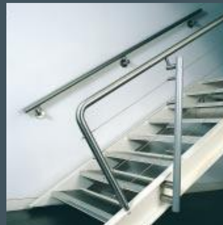
SN.4G.5G.6E.ST4 Satin Polished Stainless Steel top rail connected with Stainless Steel offset stems to Platinum NyMet® coated side fixed uprights at maximum 1200mm centres with offset Stainless Steel wire rope infill and fittings.
