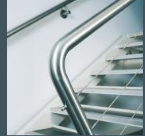
SS.1C Satin Polished Stainless Steel handrail connected at maximum 1200mm centres to Stainless Steel stem brackets with concealed fixings.
