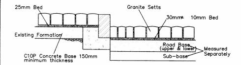
1. Joints will be grouted with 1:4 cement mortar.
