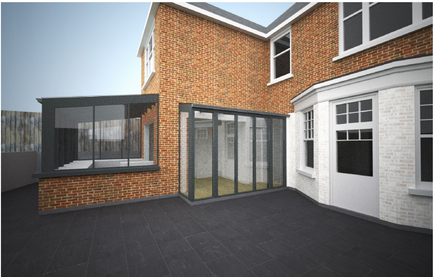
3D visualisation showing the proposed ground floor extensions in relation to the adjacent existing bay.
