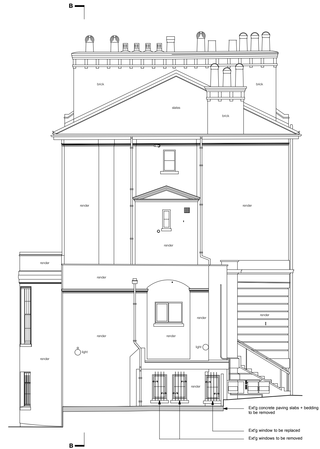
Existing side elevation
