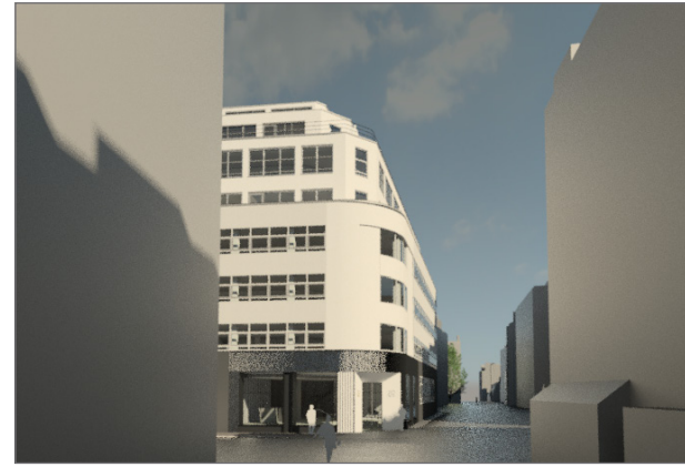
Plant screen 2000mm high, enclosure set back further from Red Lion & Sandland Streets
