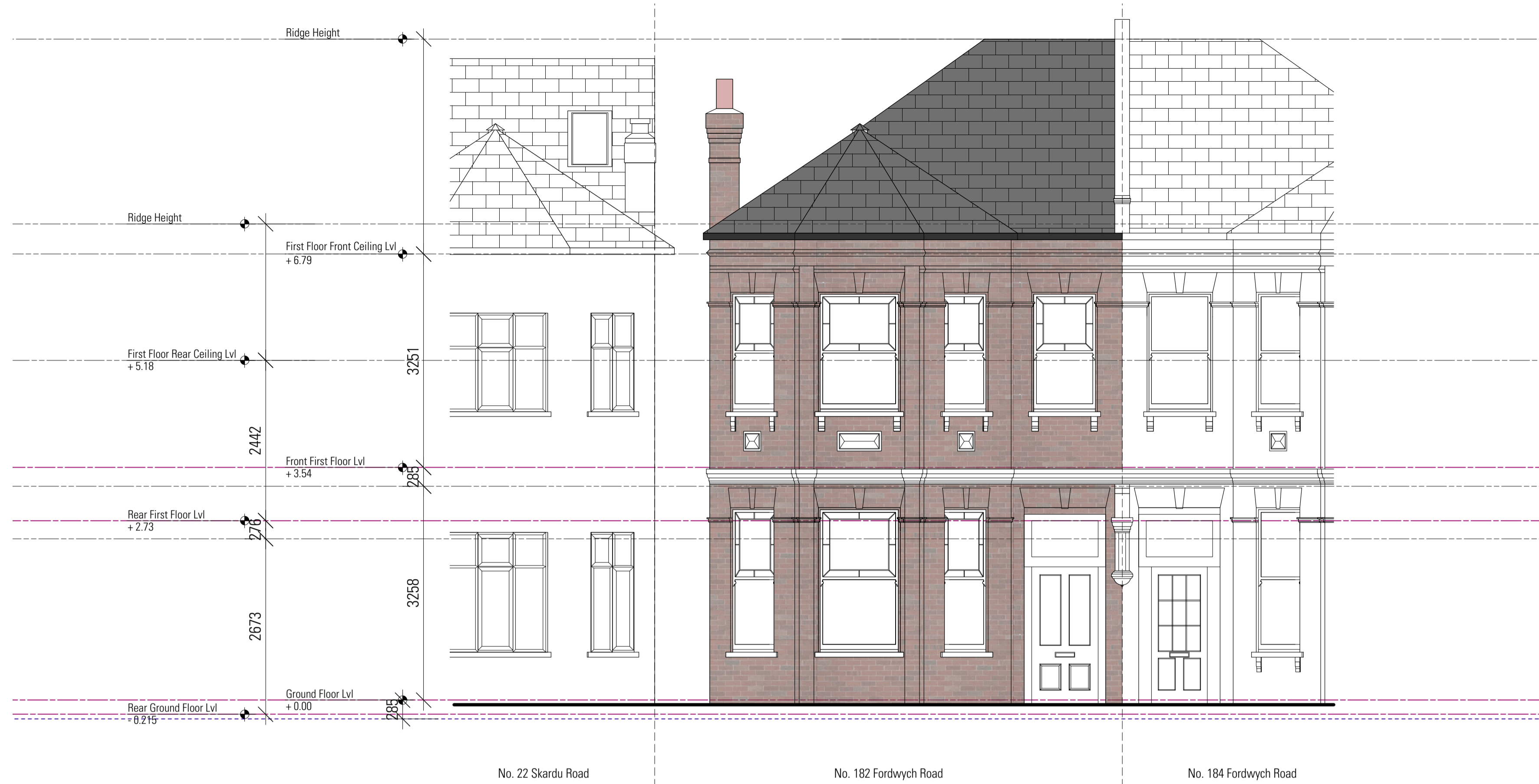
01 Existing Front Elevation Scale 1:50@A1, 1:100@A3
