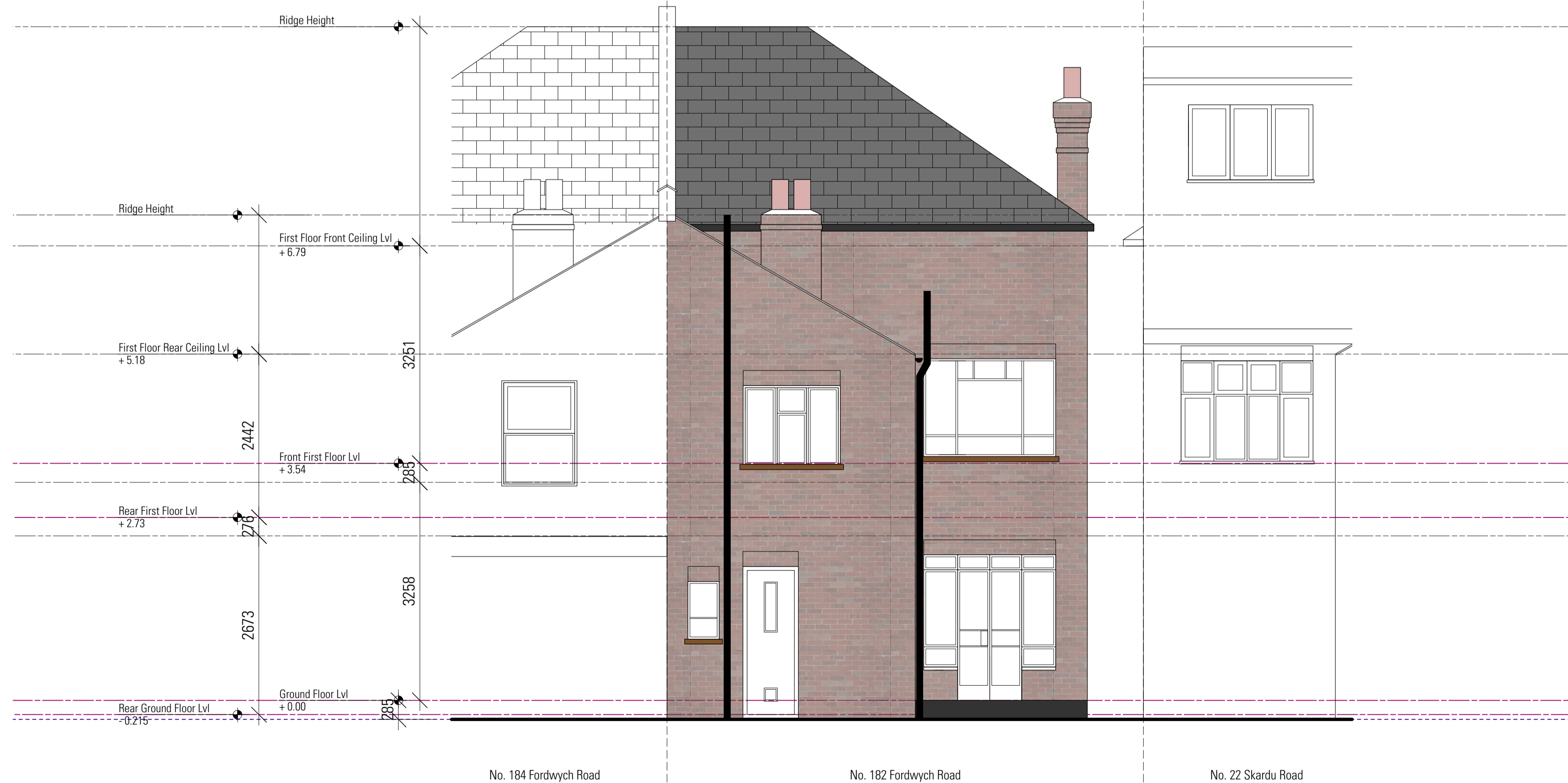
02 Existing Rear Elevation Scale 1:50@A1, 1:100@A3
