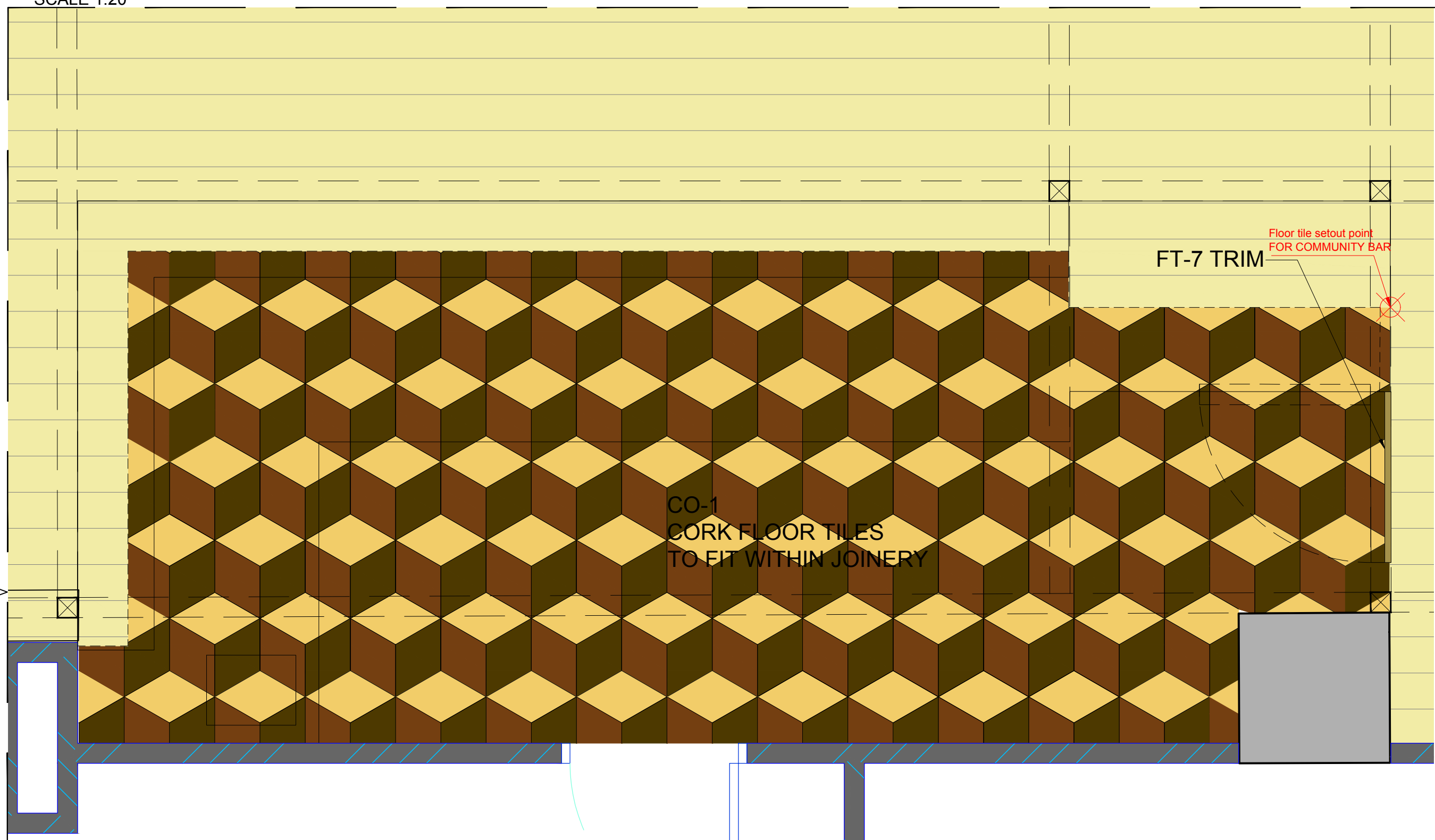
COMMUNITY BAR - FLOOR FINISHES PLAN SCALE 1:20
