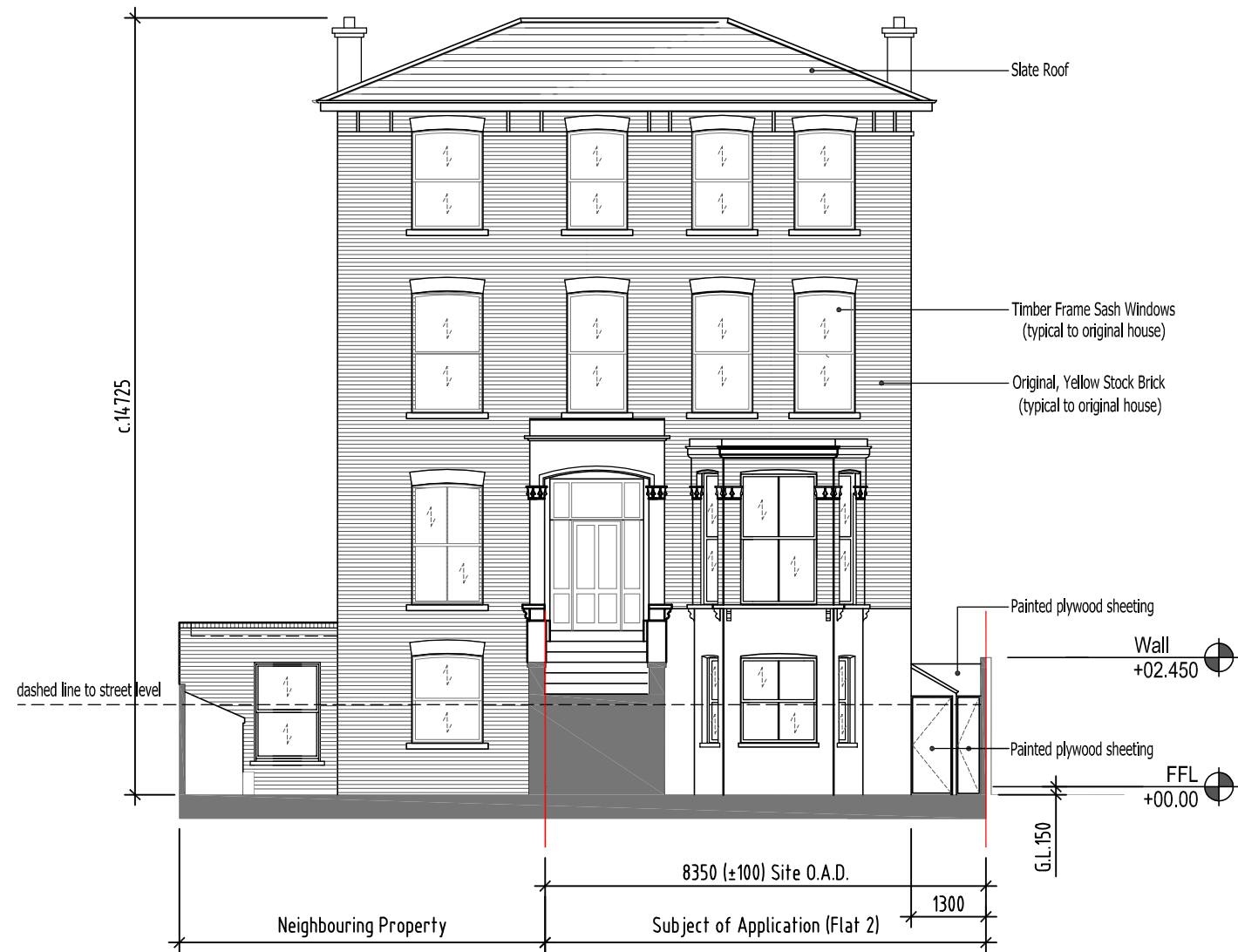
Existing Front Elevation.(West)
