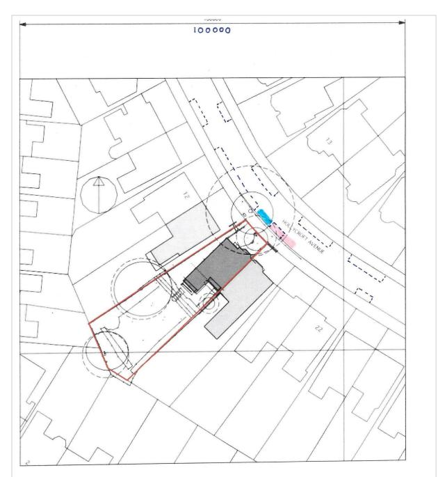
The above plan shows the proposed location of a skip shown highlighted in blue and the area which will be used for loading/unloading of materials etc highlighted in pink.
