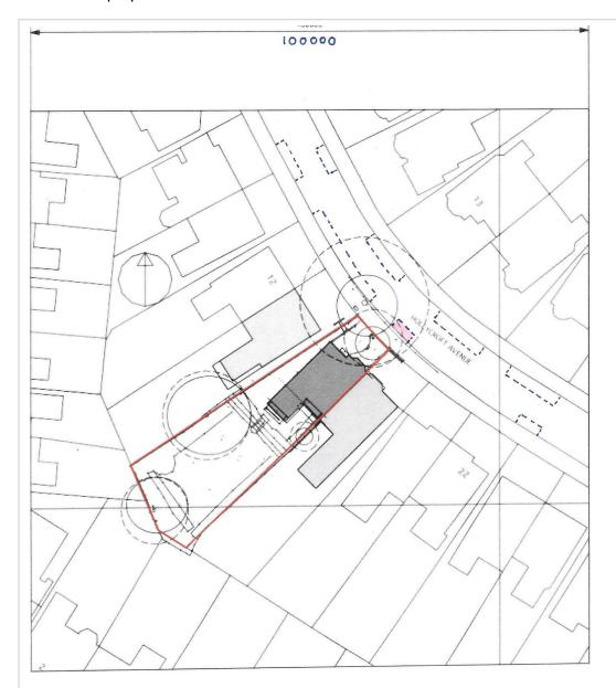
The main access to the site for materials will be via the existing cross over. There are on-street parking bays on both sides of the road, though a long gap between parking bays outside numbers 18-22. There are no cycle lanes.
