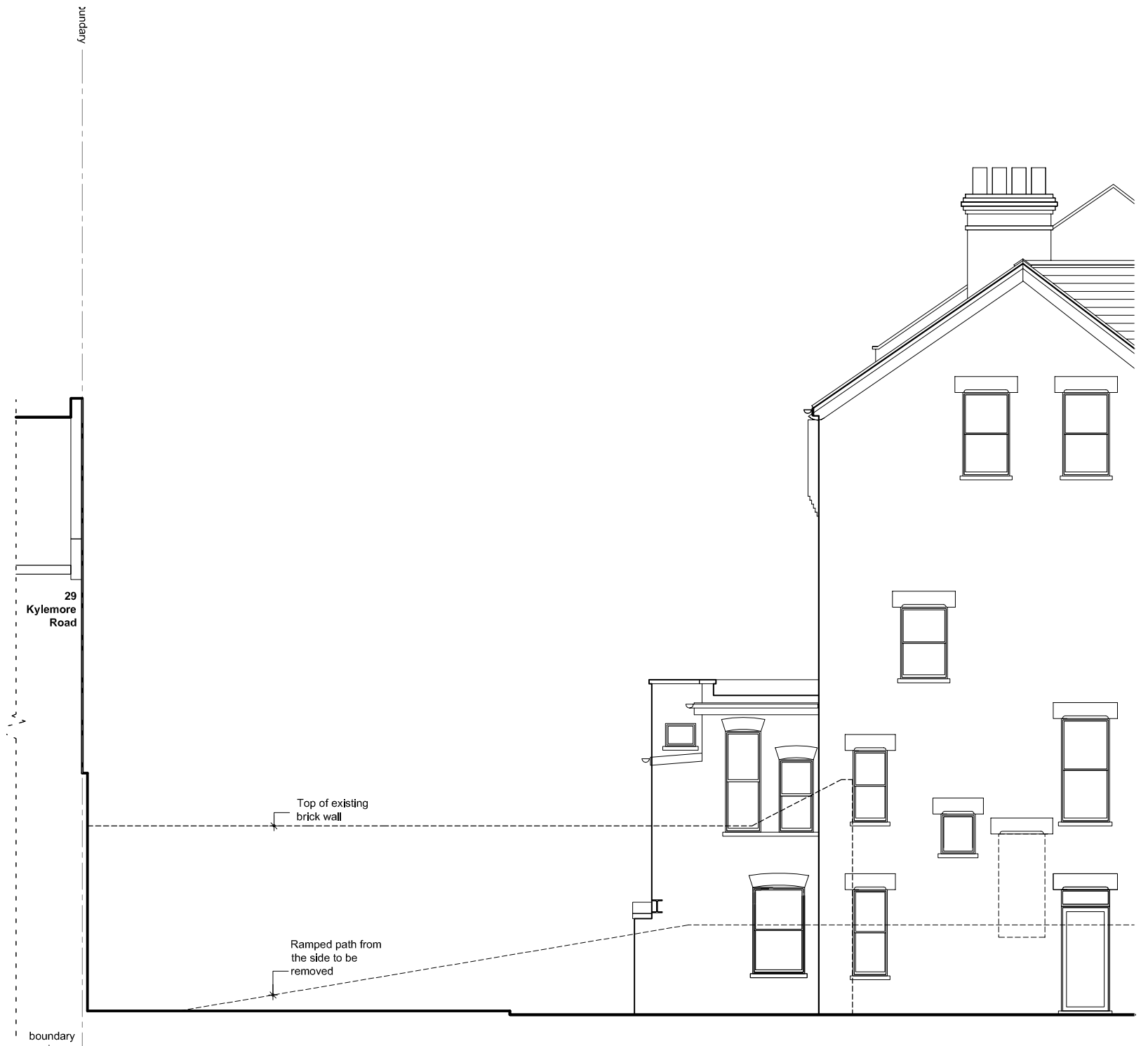
Existing Side Elevation/ Section - West
