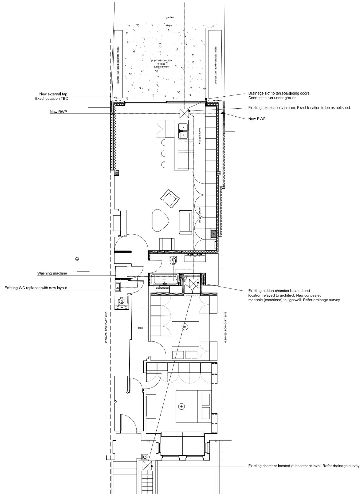
All drainage routes indicative. Contractor to establish existing drainage system and design new installation for approval of architect.
