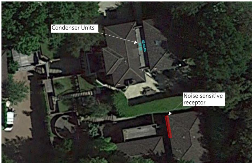
Figure 4.2: Plant location and nearest noise sensitive window
