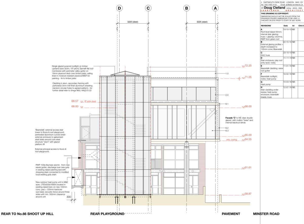
Elevation C: With 'Beanstalk': Proposed Scale 1:100 For key notes refer drawing MUL-AL(0)C01
