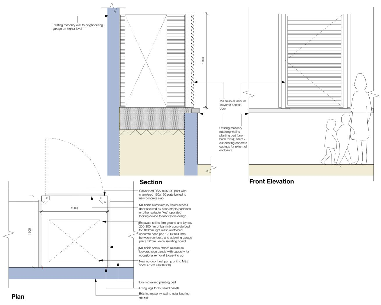
**GF External Heat Exchanger Base + Enclosure**
