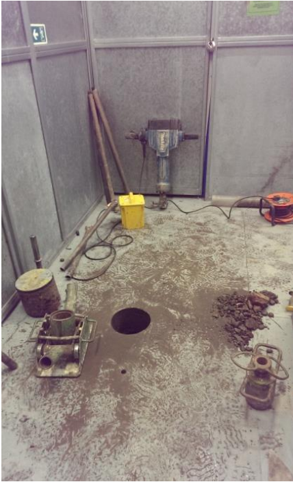
Photo 1 - Coring of borehole HM-WS1
