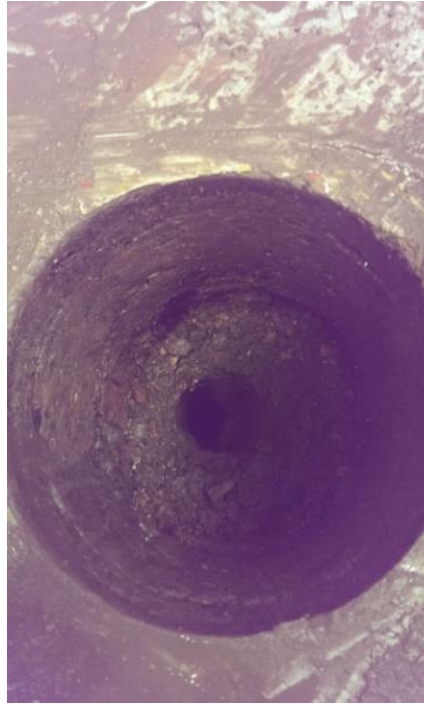
Photo 2 – View of cored slab and underlying granular Made Ground (location HM-WS2)
