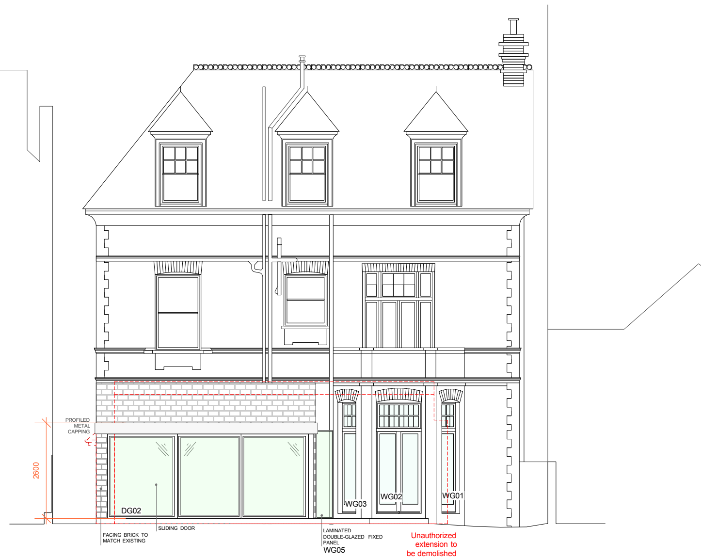
4 LANCASTER GROVE-PROPOSED/ REAR ELEVATION Scale: 1:100
