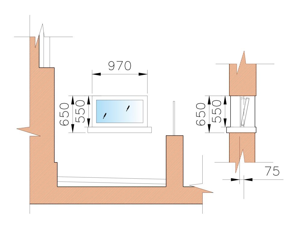
Existing wooden basement window to be removed from its hinges and the opening to made good and prepared for the new sash window. Make sire opening is not made wider or smaller.
