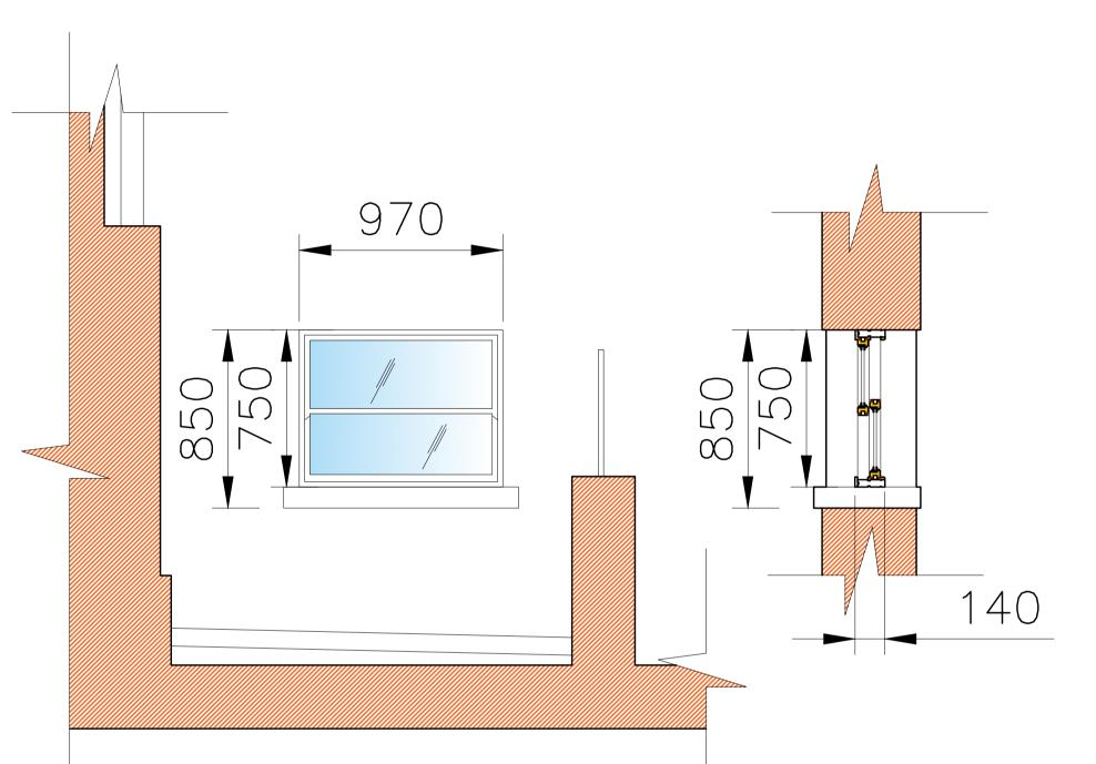
New box spring sash window with 140mm Box and parting with stop bead brushed. New window to be installed to the same location as per the original window. Size to be increased by 200mm in height (down from original window location)
