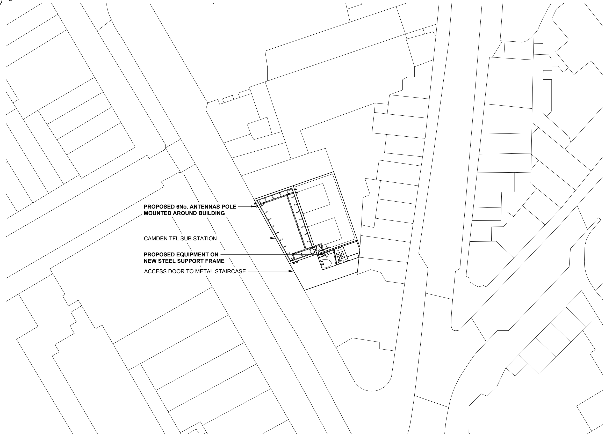
PROPOSED SITE LAYOUT PLAN (SCALE 1:500)
