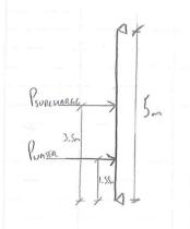
Pure =  $\frac{1}{2} \% h^2 = 0.5 \times 10 \times 5^2 = 125 \text{ kN} \otimes \frac{h}{3} = 1.55 \text{ m}$ Psurcharar =  $9 \text{ Kah} = 2.5 \times 0.5 \times 7 = 8.8 \text{ kN} \otimes \frac{h}{2} = 3.5 \text{ m}$ MEN = 139.8 kNm.
