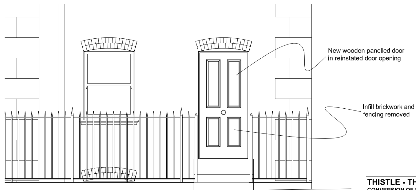
Elevation of Reinstated Door Opening As Proposed 1:25
