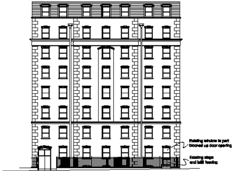
Elevation to Little Russell Street As Existing 1:100
