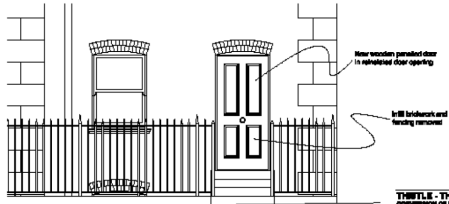
Elevation of Reinstated Door Opening As Proposed 1:25
