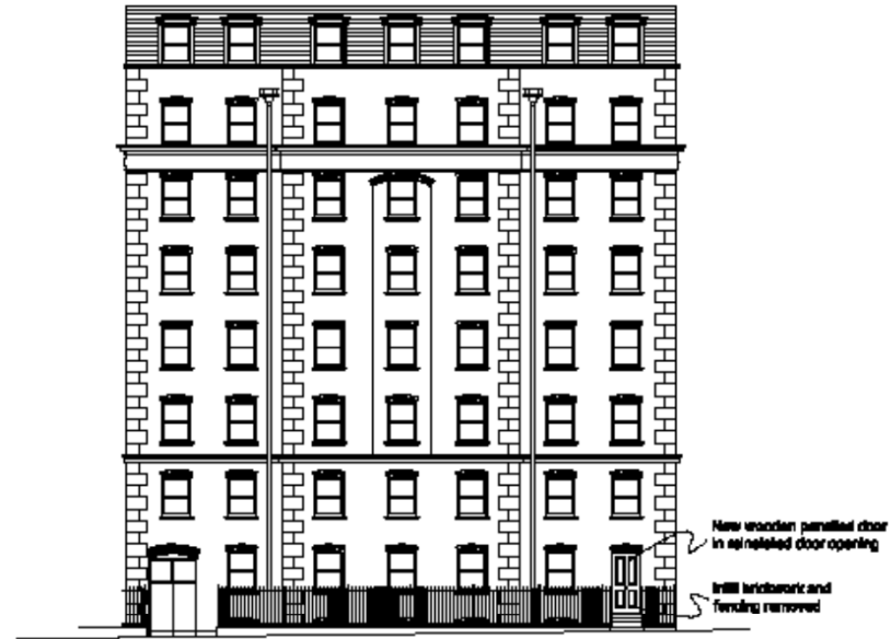
Elevation to Little Russell Street As Proposed 1:100
