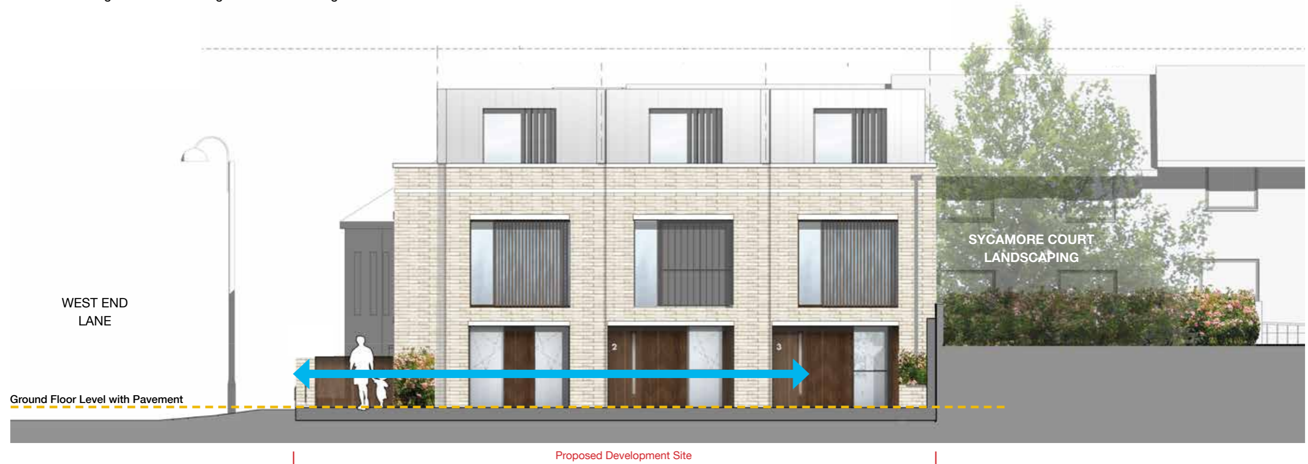
Section AA: Diagram Section through Entrance showing Level Access
